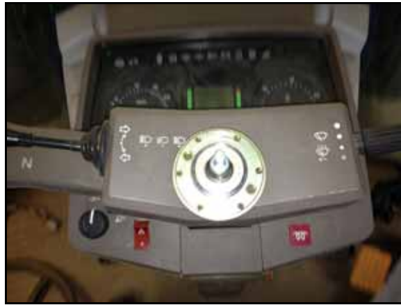
FIGURE 7. Female Spline Adapter Installed on Steering Column
