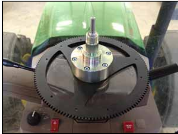
FIGURE 12. Male Spline Adapter Assembly Installed
