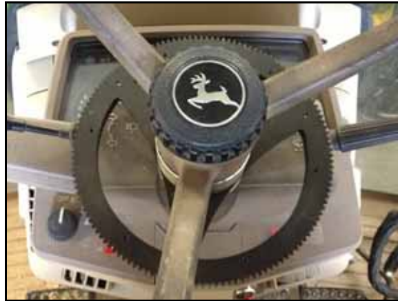
FIGURE 16. Steering Wheel Cap Reinstalled
