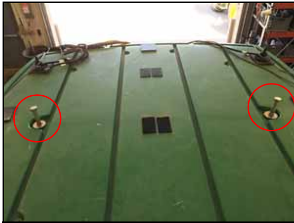
FIGURE 1. Machine's Bolts and Washers to be Removed
