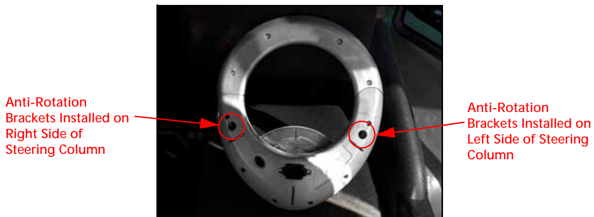
FIGURE 21. Anti-Rotation Pin Installation Locations
