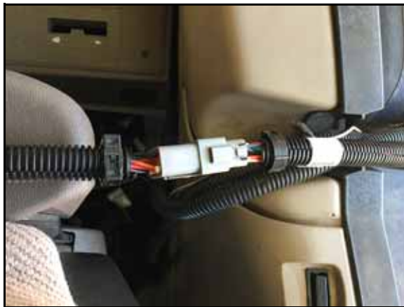
FIGURE 10. RS1 Tee Cable Connected to RS1 MD Cable
