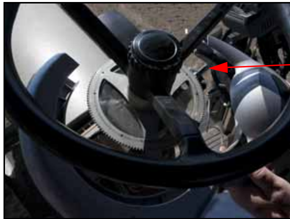
FIGURE 22. Anti-Rotation Pin Installed in Bracket Assembly
