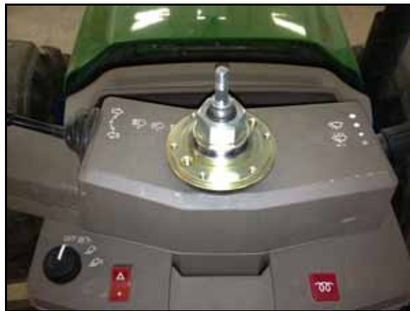
FIGURE 8. Machine's Steering Wheel Nut Installed
