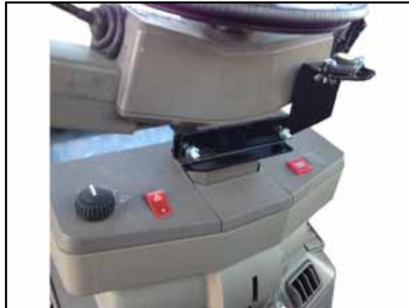
FIGURE 20. Bracket Installed on Steering Column
