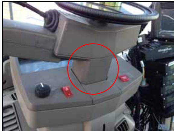
FIGURE 17. Bracket Installation Location
