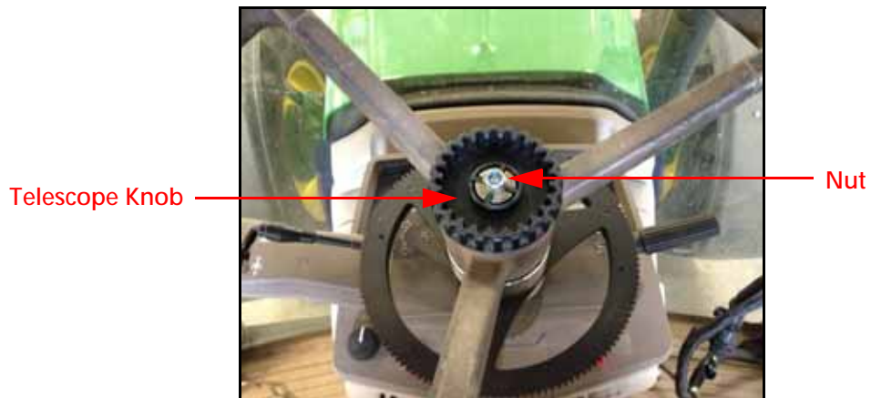
FIGURE 15. Telescope Knob and Nut Reinstalled
