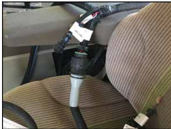
FIGURE 12. RS1 MD Connected to Console Cable
