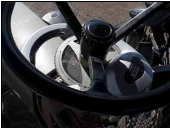
FIGURE 23. Mechanical Drive Installed
