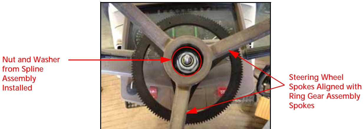
FIGURE 13. Steering Wheel Placement
