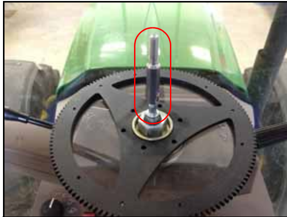
FIGURE 11. Telescope Adapter Assembly Installed
