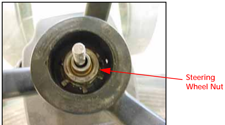
FIGURE 4. Machine's Telescope Knob Removed
