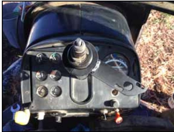
FIGURE 7. Anti-Rotation Bracket Installed
