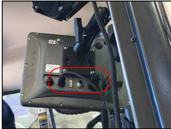
FIGURE 13. Console Cable Connected to Console
