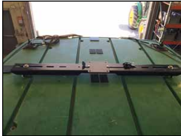
FIGURE 3. RS1 Crossbar Assembly Installed
