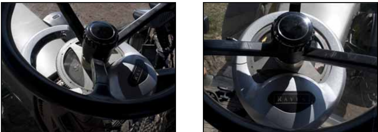
FIGURE 19. Mechanical Drive Installed
