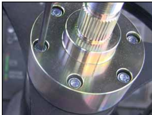
FIGURE 12. Male Spline Assembly Installed
