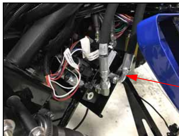
FIGURE 3. Pressure Hose Installed on AutoBoom Valve
