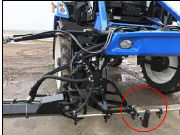
FIGURE 5. Center Rack Sensor Mounting
