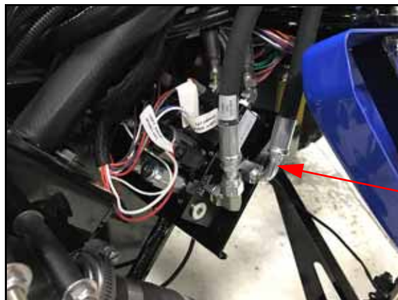
FIGURE 3. Pressure Hose Installed on AutoBoom Valve
