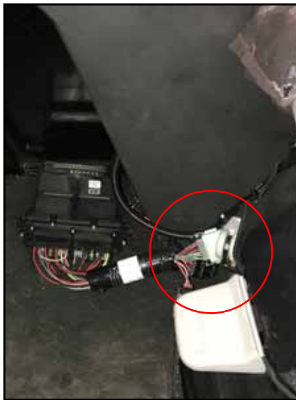
FIGURE 4. Valve Harness Connected to Node Harness
