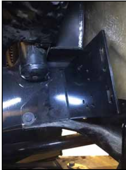
FIGURE 6. SmarTrax Valve Mounting Bracket Installed
