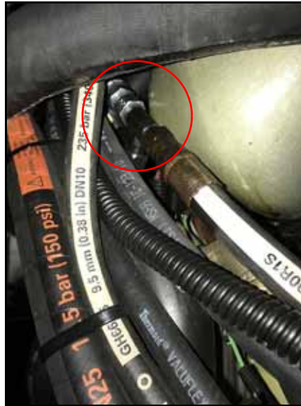
FIGURE 10. Machine's Pressure Hose Connected to Installed Pressure Hose
