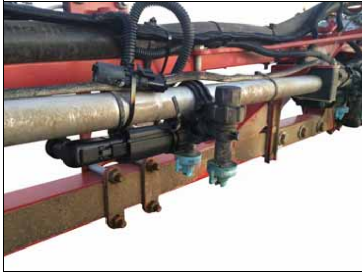
FIGURE 3. Modified Nozzle Control Valve Installation
