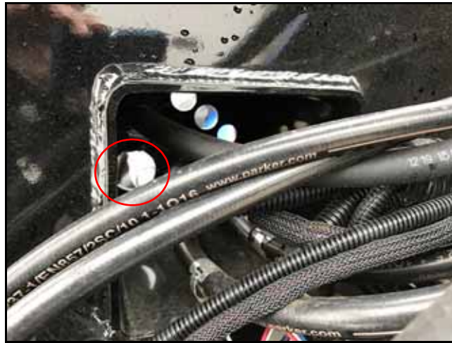
FIGURE 2. Bulkhead Location (Front View)
