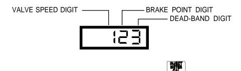
To change the Valve Cal setting, depress the key labelled **5** for 5 seconds. The display will show the current valve calibration number. Enter a new valve calibration number if desired.
