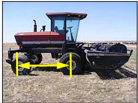
Wheel base measurement taken with wheels reversed and not in the straight line operation position.
