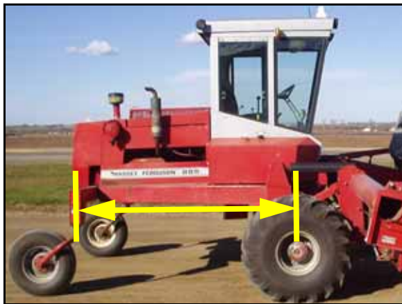
Wheel base measurement taken from pivot point instead of the center of the front wheel.
