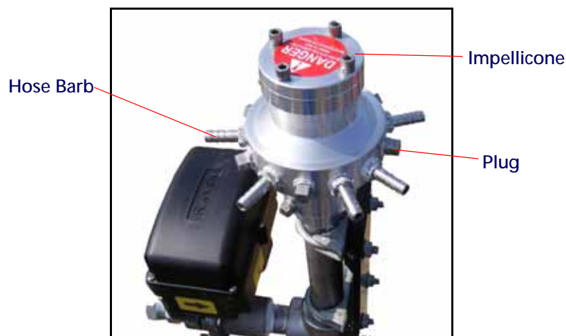
FIGURE 1. Impellicone with Alternating Barbs and Plugs Installed
