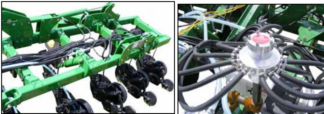
FIGURE 7. Liquid Applicator Lines Connected to Impellicone
