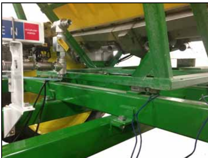
FIGURE 6. Incorrect Installation (Outlet Tee Not Clearing Bin Support)
