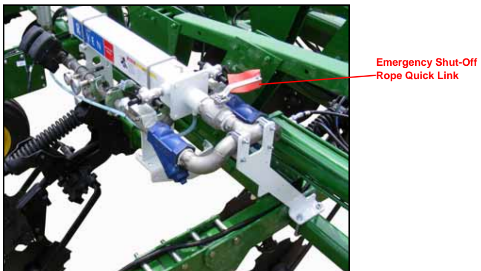
FIGURE 6. Emergency Shut-off Rope Installation
