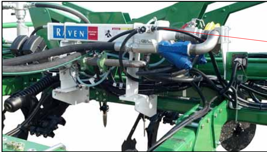
FIGURE 5. Vapor Line Installation.
