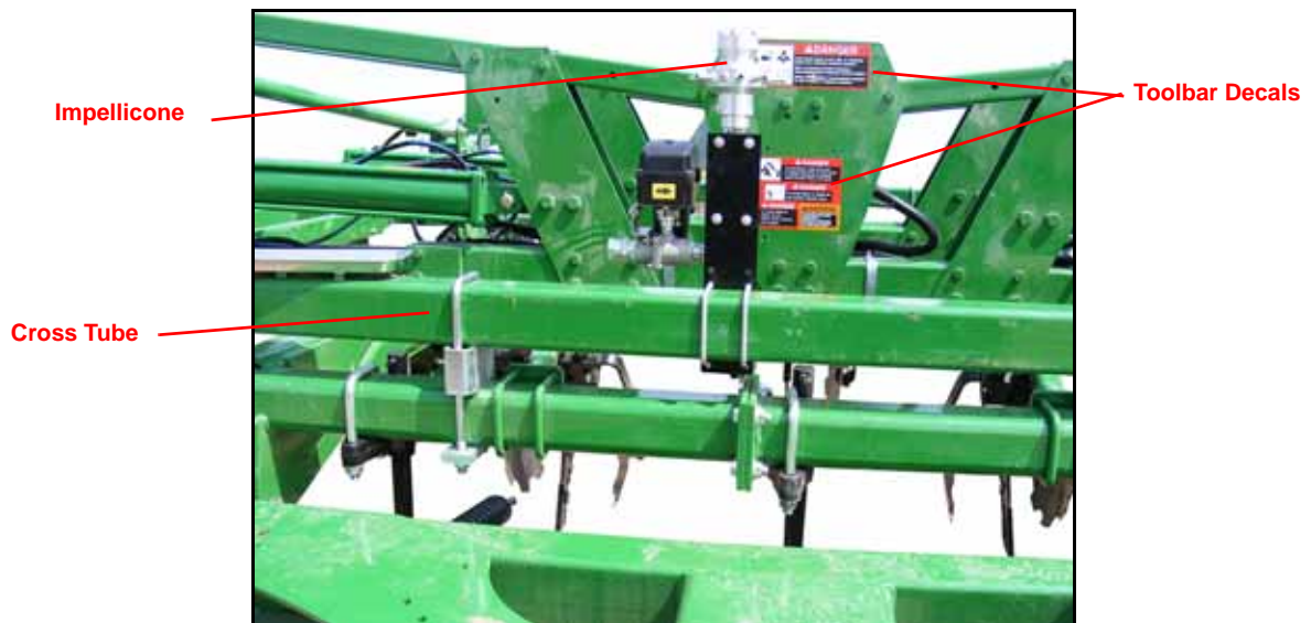
FIGURE 5. Installed Impellicone with Visible Decals
