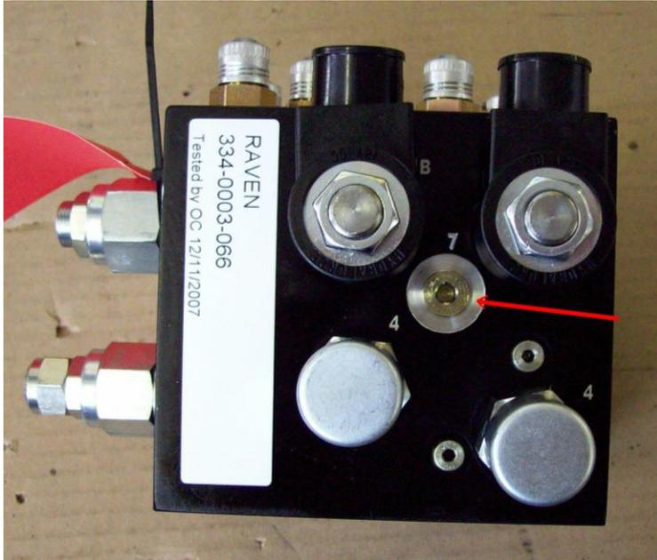
**Note:** None of the 334-0003-056 valves have been reworked to have the hydraulic fix done externally. Any of the valves shown here that do not have a internal hydraulic fix will require the 117-0191-010 external hydraulic fix. Any valves older than these will not work with a yaw style system.
