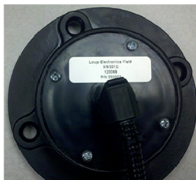
New Sensor Example Silver Sticker with Date, Product and Serial Number or engraved with a Y
