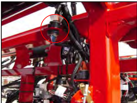
FIGURE 14. Cabo do Chicote AutoBoom Instalado
