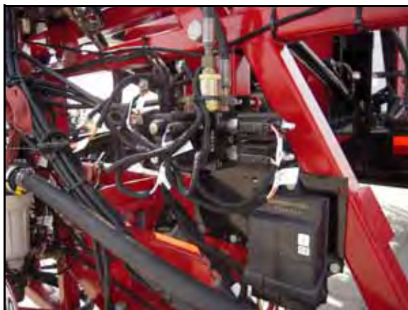
FIGURE 10. Nodo AutoBoom Instalado
