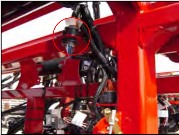
FIGURE 11. Cabo do chicote AutoBoom Instalado
