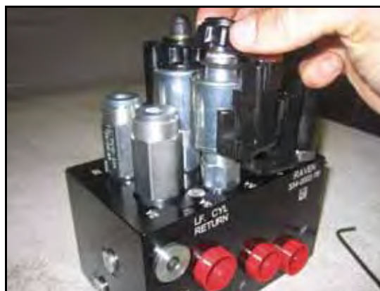
FIGURE 6. Mola Reinstalada na Válvula AutoBoom
