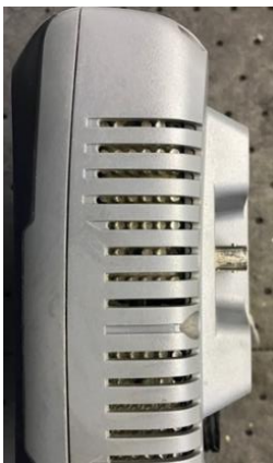
Non-Repairable Heat Sink can be seen through vent openings
