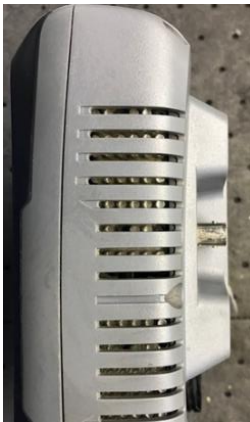
Non-Repairable Heat Sink can be seen through vent openings
