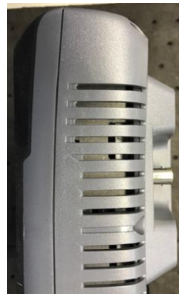
Limited Repair Flat metal can be seen through vent openings.
