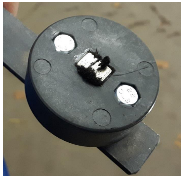
Figure 33 Dirty wheel angle sensor magnet.
