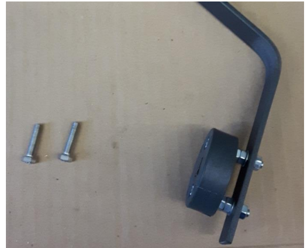
Figure 32 Wheel angle sensor disc mounted with spacers.
