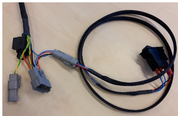
Figure 18 Master switch connected to the terminal harness.
