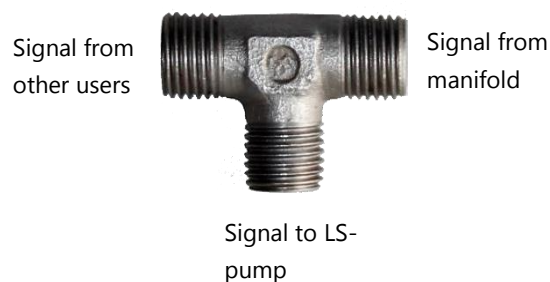
Figure 5 Top view of shuttle valve for mounting in the load sense line.
