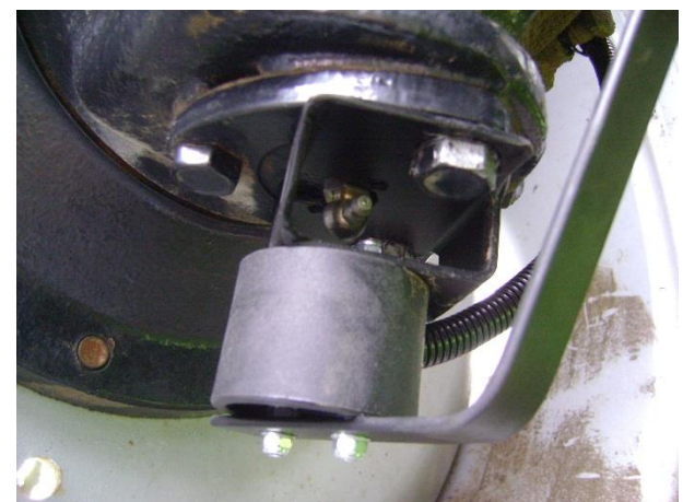
Figure 26 Stub axle with grease nipple.
