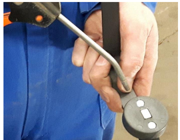
Figure 34 Cleaning wheel angle sensor magnet.
