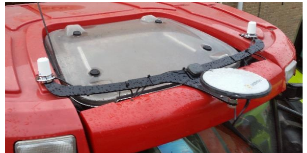
Figure 47 Case New Holland with GPS-antenna, GPS patch antenna and two GPRS/UMTS antenna's.
