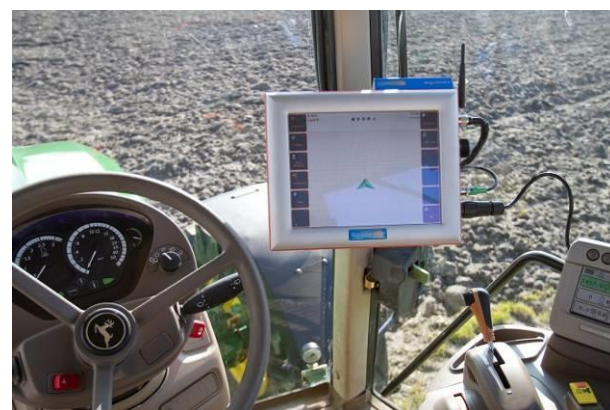
Figure 52 GeoStar terminal mounted to ISO attachment of A-pillar.
