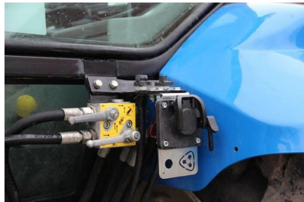
Figure 12 IBBC bracket with connector.
