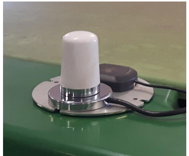
Figure 48 GPRS/UMTS-antenna and GPS patch antenna on a metal bracket.
