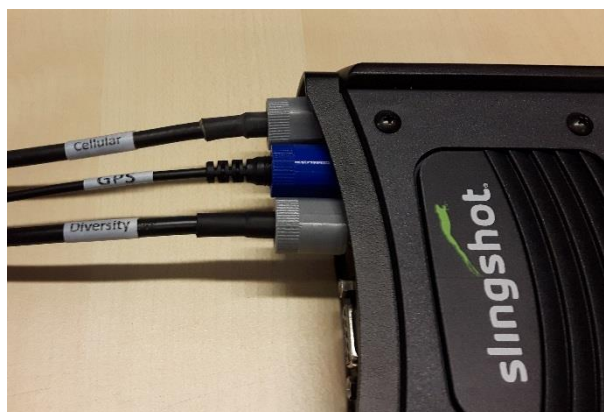
Figure 49 Antenna cables with labels and SMA-grip set.
