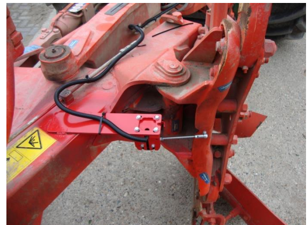
Figure 4 Angle sensor mounted to plough without moveable width beam.
