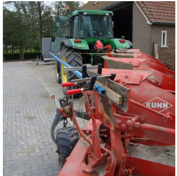
Figure 18 Measuring the plough width
