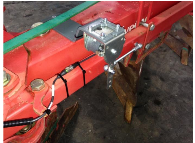
Figure 3 Angle sensor mounted to moveable width beam
