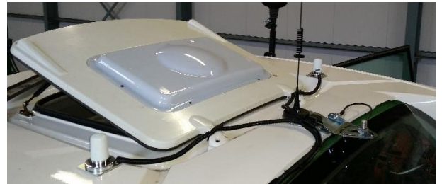
Figure 9 Mounting antennes on the roof
