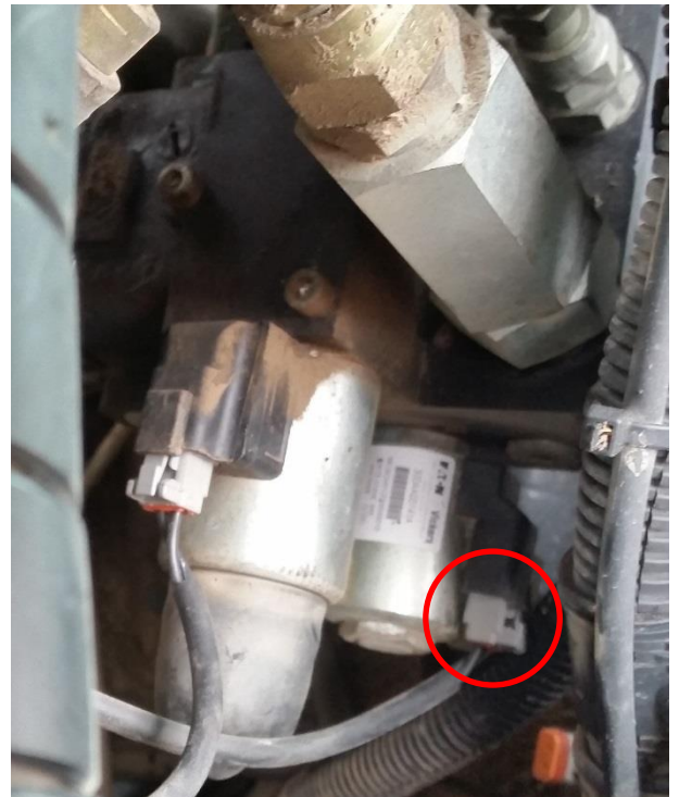
Figure 5 Connection of the STU – NH intellisteer harness on the CNH lock valve
