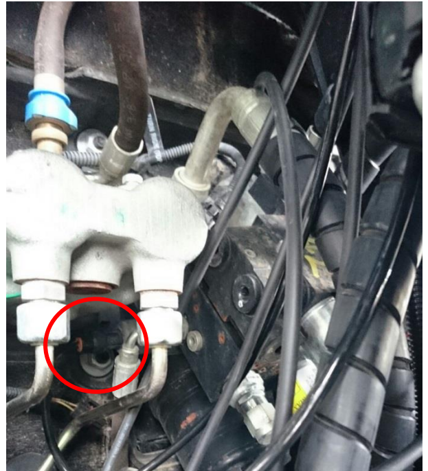
Figure 6 Connection of the STU – NH intellisteer harness on the CNH pressure sensor
