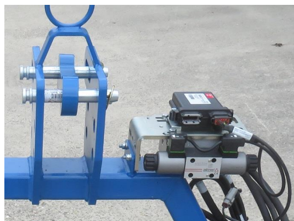
Figure 3 Manifold and STU mounted on Side-Shift frame
