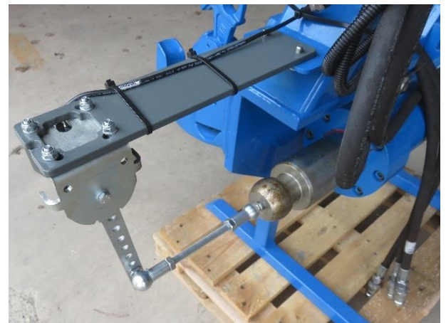
Figure 9 Mounting angle sensor Side-shift adapter frame
