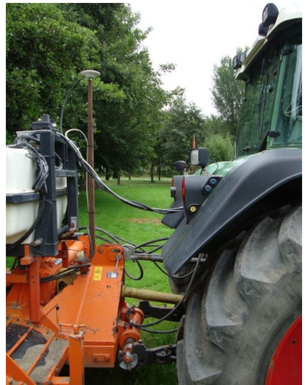
Figure 11 GPS-antenna position on Side-Shift steering
