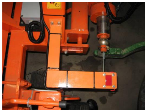
Figure 7 Mounting angle sensor Side-shift steering top view
