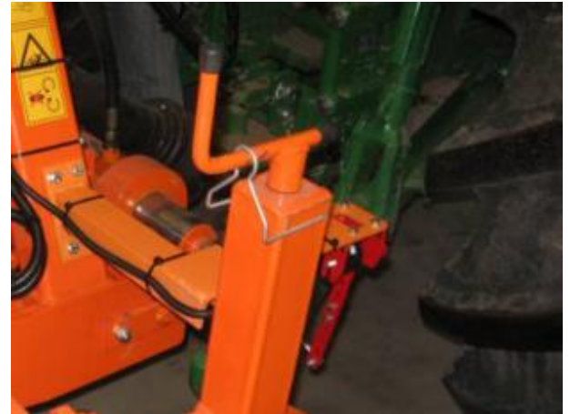
Figure 8 Mounting angle sensor Side-Shift steering side view
