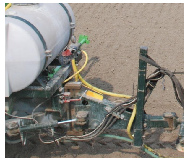
Figure 10 Mounting angle sensor drawbar steering
