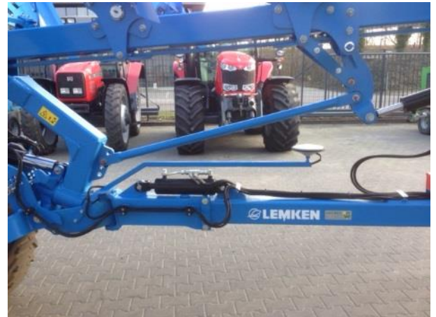
Figure 14 GPS-antenna on semi-mounted reversible plough in transport position
