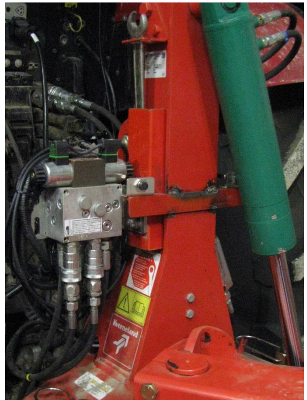
Figure 13 Alternative mounting position for proximity sensors
