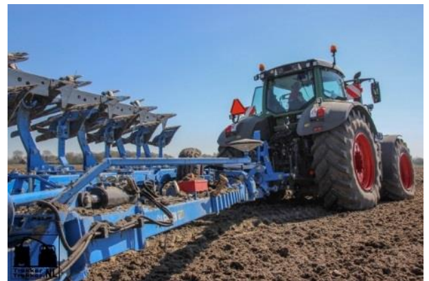
Figure 15 GPS-antenna mounted on semi-mounted reversible plough in ploughing position
