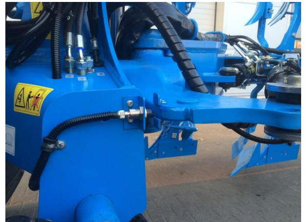
Figure 12 Proximity-sensors mounted on the rear mounted three-point linkage of the plough
