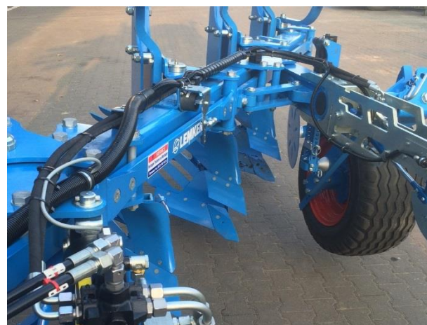
Figure 17 Guiding of cabling
