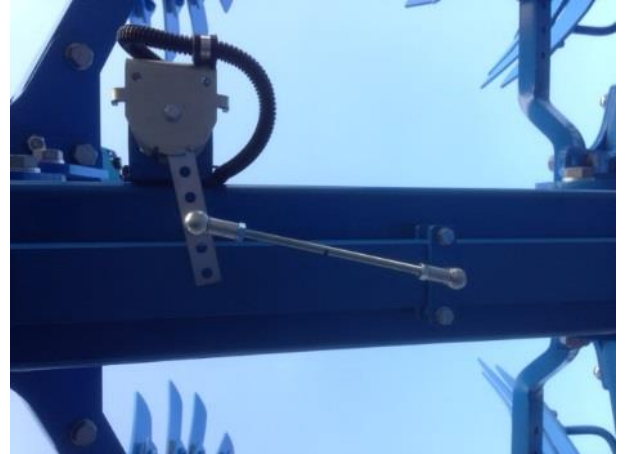
Figure 3 Angle sensor mounted on plough with plough width regulation beam
