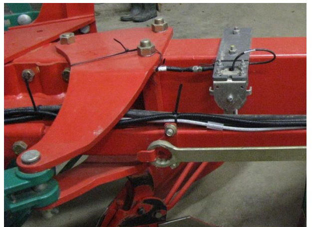
Figure 4 Angle sensor bracket straight clamped to the frame with two pieces of threaded rod
