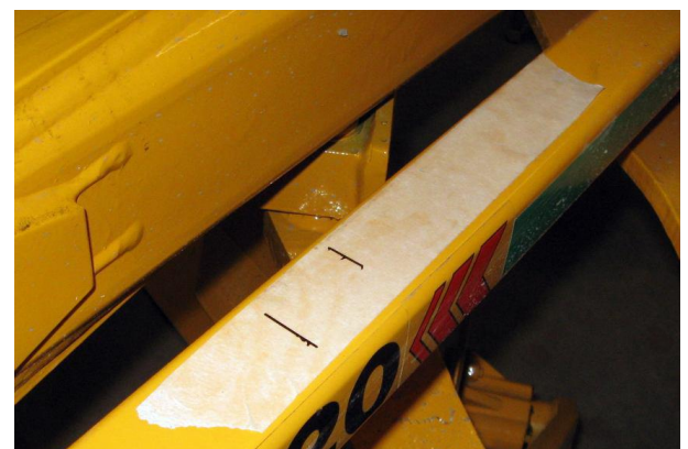
Figure 5 Angle sensor range on width regulation beam
