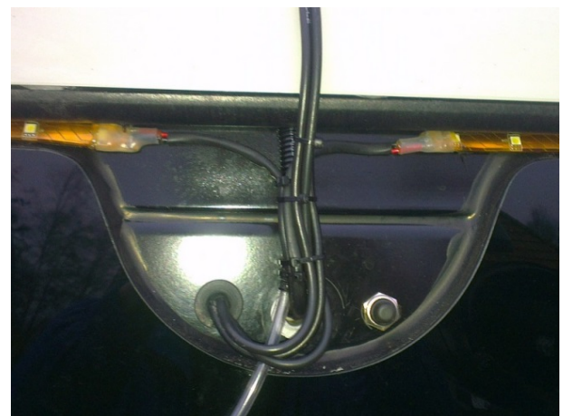
Figure 34 Radio cable at the back of the cabin (Outside)
