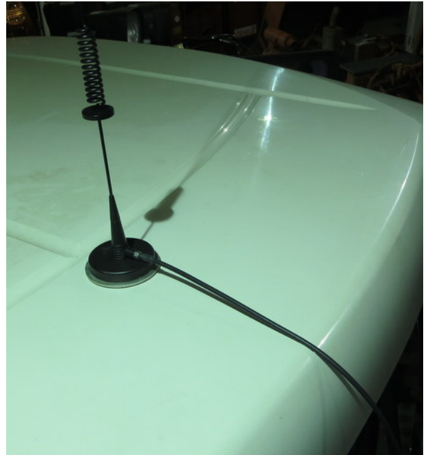
Figure 33 Radio antenna mounted on Condor roof
