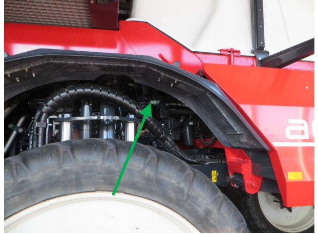
Figure 21 Location of the split manifold on an Iveco engine
