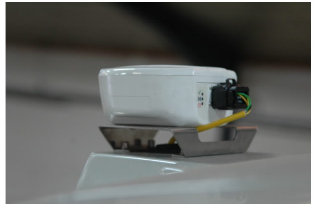
Figure 30 Novatel Smart-AG Egnos mounted on Condor roof
