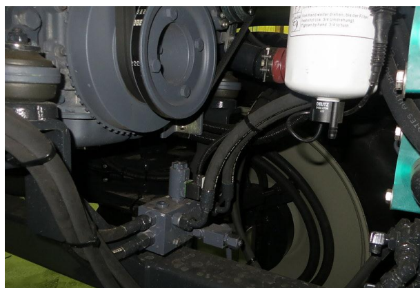
Figure 18 Split Manifold at the front of the engine (Only Deutz engines)
