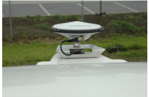
Figure 32 RTK GPS Antenna mounted on top of the Condor roof
