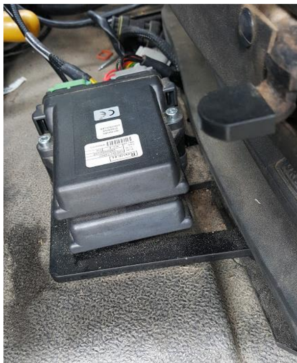
FIGURE 33 DYNAMIQ ISO AND STU MOUNTED NEXT TO THE SEAT.
