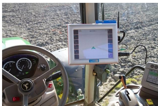
FIGURE 37 GEOSTAR TERMINAL MOUNTED TO ISO ATTACHMENT OF A-PILLAR.
