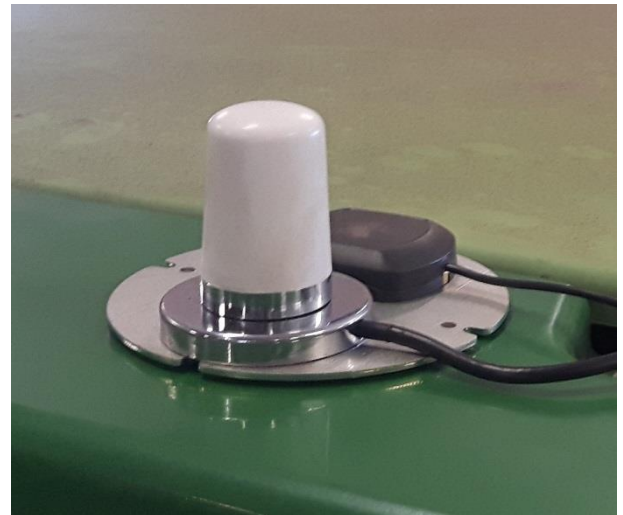
FIGURE 30 GPRS/UMTS-ANTENNA AND GPS PATCH ANTENNA ON A METAL BRACKET.
