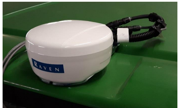
FIGURE 26 RAVEN 600S ANTENNA ON A CABIN.
