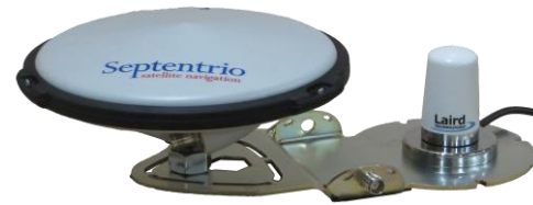
FIGURE 32 GPS ANTENNA BRACKET WITH A LAIRD UMTS ANTENNA.
