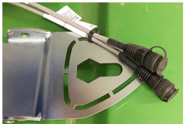
FIGURE 27 CABLES TO THE RAVEN 600S ANTENNA.
