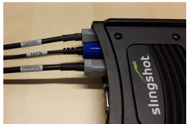
FIGURE 31 ANTENNA CABLES WITH LABELS AND SMA-GRIP SET.
