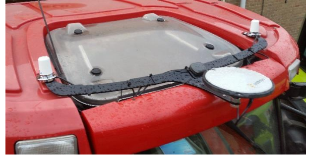
FIGURE 29 CASE NEW HOLLAND WITH GPS-ANTENNA, GPS PATCH ANTENNA AND TWO GPRS/UMTS ANTENNA'S.
