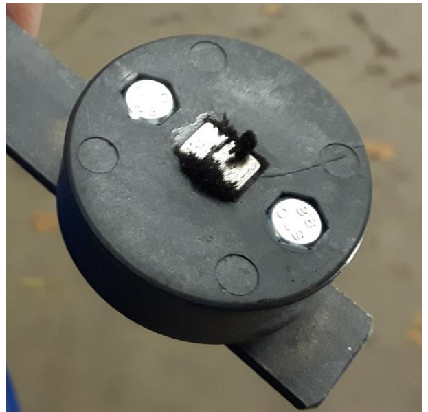
FIGURE 16 DIRTY WHEEL ANGLE SENSOR MAGNET.
