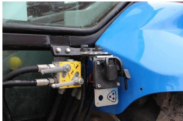
FIGURE 2 IBBC BRACKET WITH CONNECTOR.
