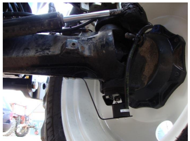
FIGURE 8 STEERING ANGLE SENSOR ON NEW HOLLAND.
