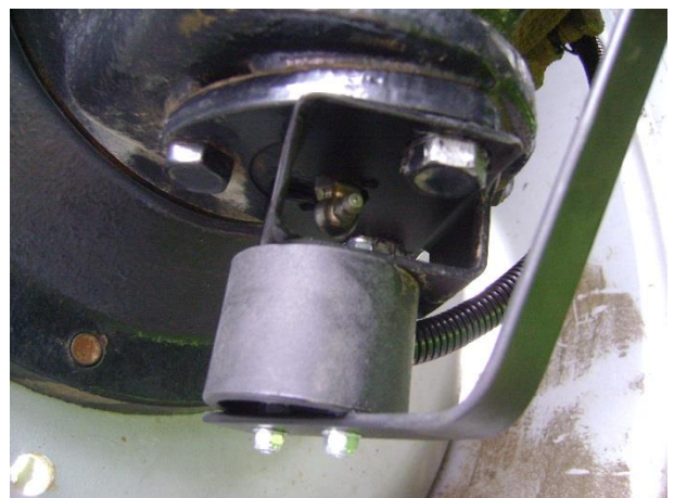
FIGURE 9 STUB AXLE WITH GREASE NIPPLE.
