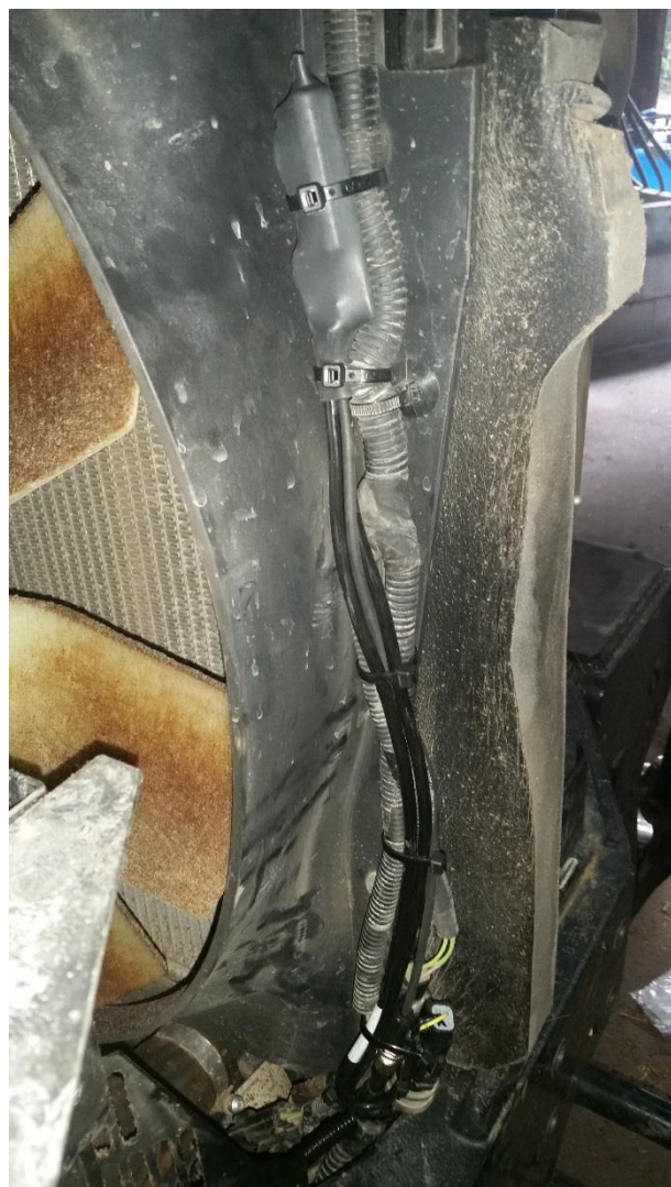
FIGURE 4 SPY CABLE MOUNTED ON A CNH TRACTOR.
