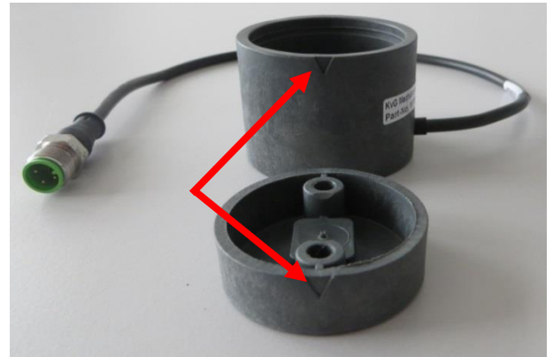
Figure 24 Triangular markings on the 12V wheel sensor.
