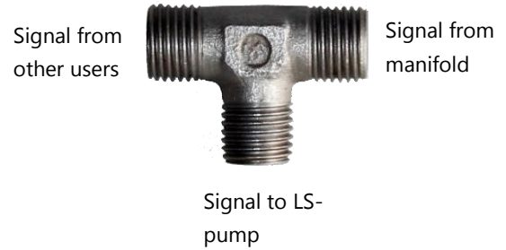
Figure 5 Top view of shuttle valve for mounting in the load sense line.
