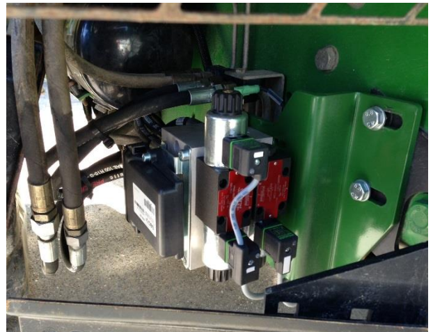
Figure 2 Mounted manifold and steering controller.
