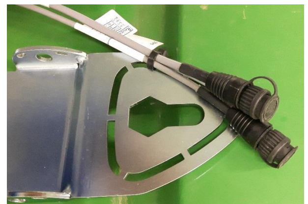
Figure 44 Cables to the Raven 600S antenna.
