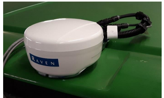
Figure 43 Raven 600S antenna on a cabin.
