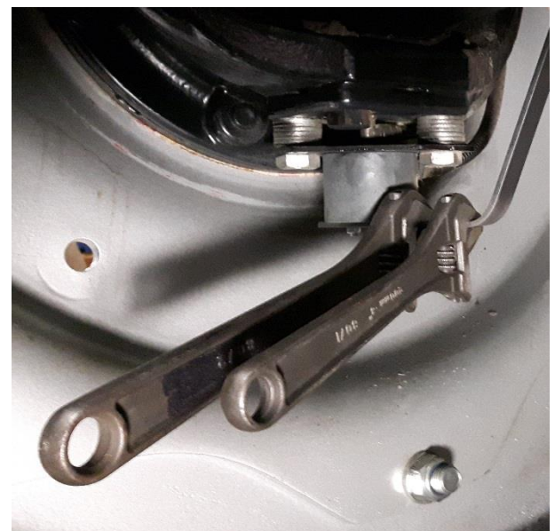
Figure 30 Bend the strip with the help of two Bahco's.
