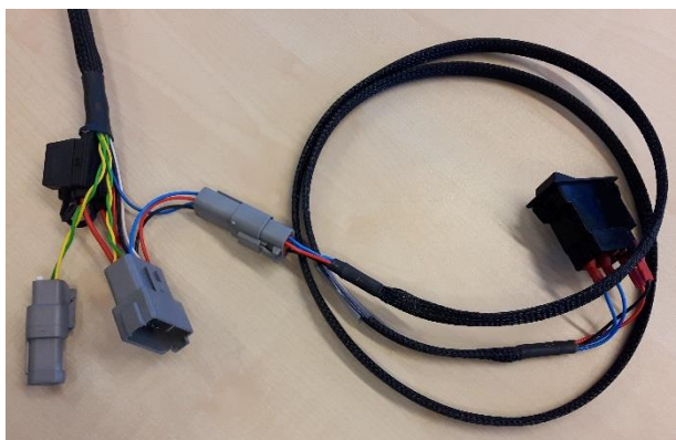
Figure 18 Master switch connected to the terminal harness.
