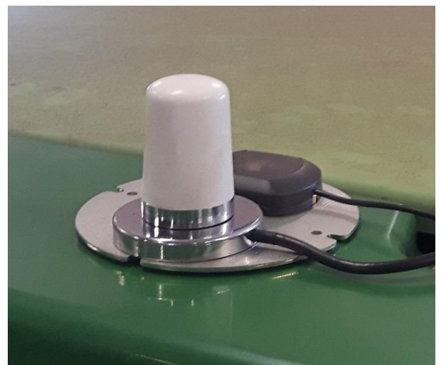
Figure 15 GPRS/UMTS-antenna and GPS patch antenna on a metal bracket.
