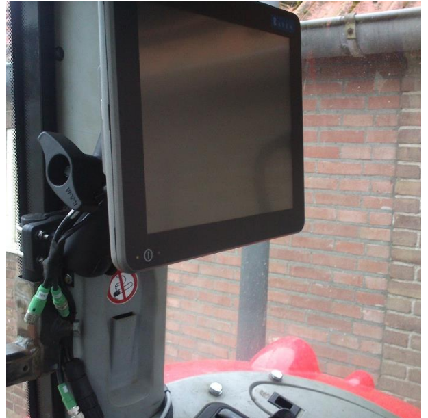
Figure 18 Viper 4 mounted with pipe bracket.
