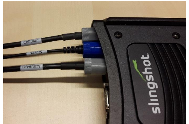
Figure 16 Antenna cables with labels and SMA-grip set.
