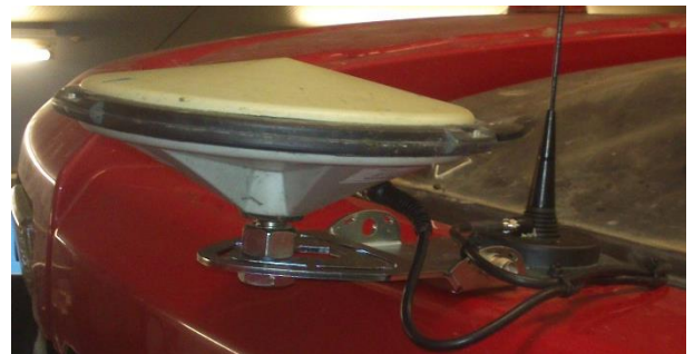
Figure 8 Standard GPS-antenna bracket + UNC bolt and nut mounted on a roof
