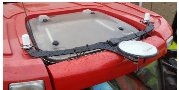
Figure 14 Brand specific bracket with GPS-antenna, GPS patch antenna and two GPRS/UMTS antennas.
