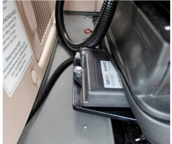
Figure 17 DynamIQ ISO on a mounting plate.
