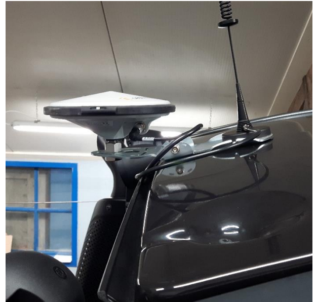
Figure 7 Standard GPS-antenna bracket + UNC bolt and nut mounted on a roof
