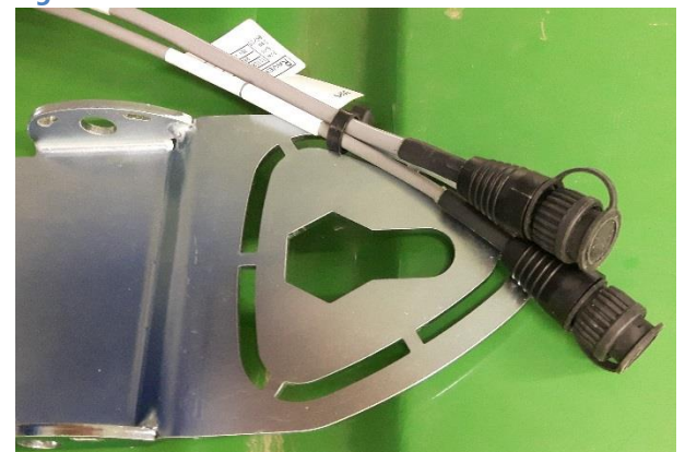
Figure 10 Cables to the Raven 600S antenna.
