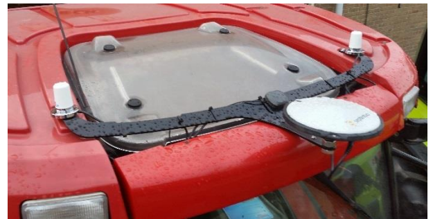
Figure 13 Brand specific bracket with GPS-antenna, GPS patch antenna and two GPRS/UMTS antennas.
