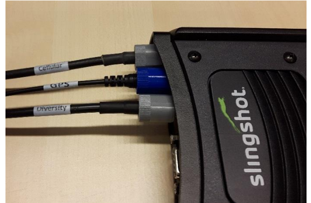
Figure 15 Antenna cables with labels and SMA-grip set.
