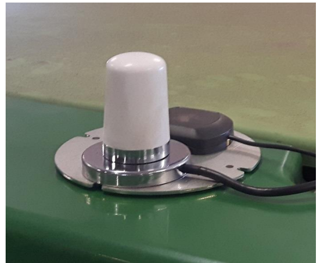
Figure 14 GPRS/UMTS-antenna and GPS patch antenna on a metal bracket.
