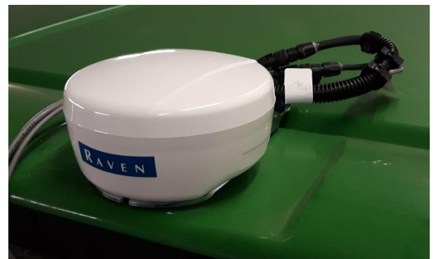
Figure 9 Raven 600S antenna on a cabin.
