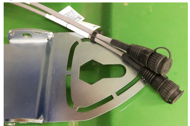
Figure 13 Cables to the Raven 600S antenna.
