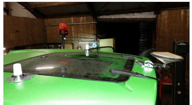
Figure 15 Brand specific bracket with GPS-antenna, GPS patch antenna and two GPRS/UMTS antennas.
