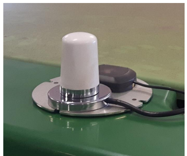
Figure 16 GPRS/UMTS-antenna and GPS patch antenna on a metal bracket.
