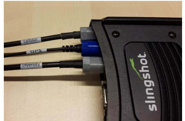
Figure 17 Antenna cables with labels and SMA-grip set.
