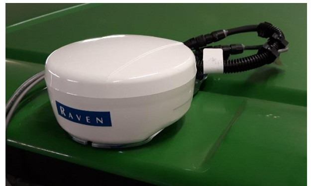
Figure 12 Raven 600S antenna on a cabin.
