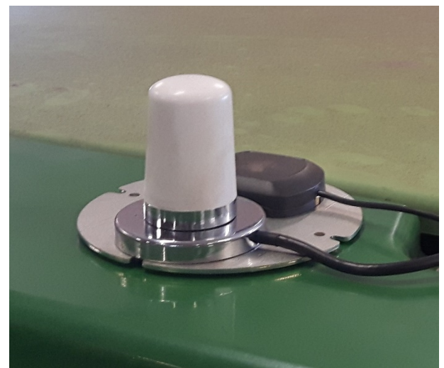
Figure 13 GPRS/UMTS-antenna and GPS patch antenna on a metal bracket.
