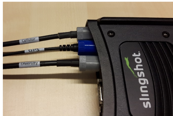
Figure 14 Antenna cables with labels and SMA-grip set.
