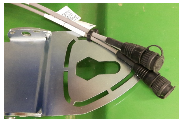
Figure 10 Cables to the Raven 600S antenna.
