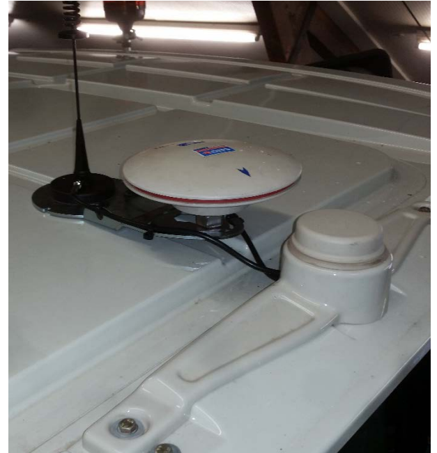
Figure 7 Standard GPS antenna bracket + UNC bolt and nut mounted on a Claas roof.
