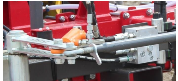
Figure 6 Hydraulic manifold mounted
