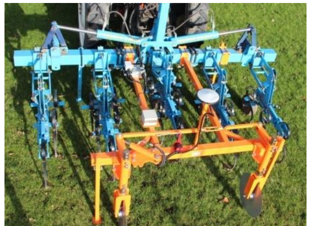
Figure 18 Dual disc steering with mechanical track rod on a retractable implement
