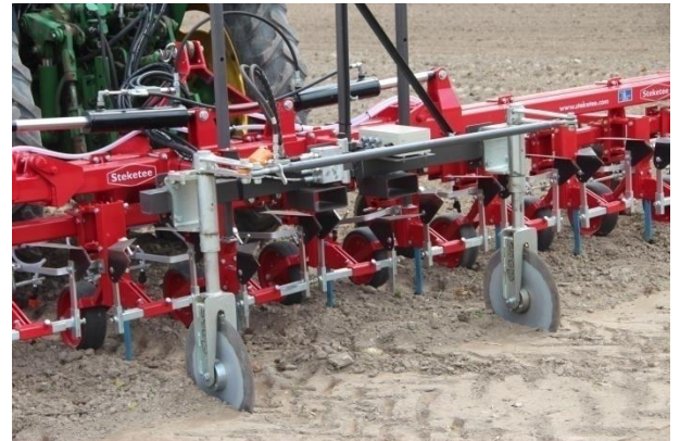
Figure 17 Dual disc steering with mechanical track rod
