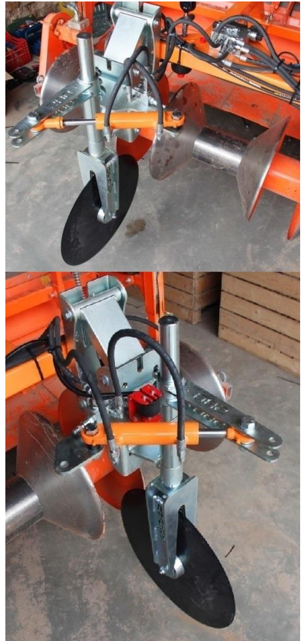
Figure 19 Dual disc steering with hydraulic track rod
