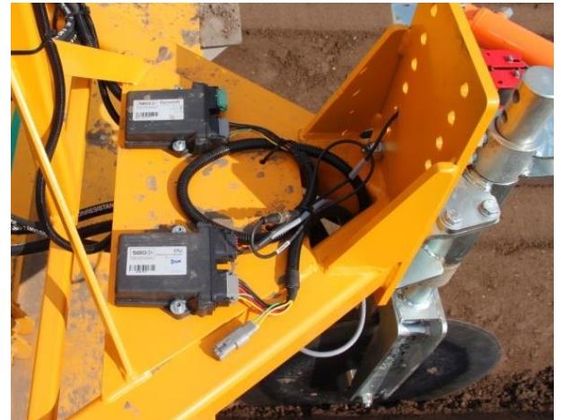
Figure 7 Steering Controller and DynamIQ
