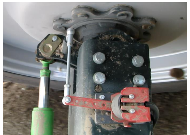
Figure 27 Angle sensor mounted at wheel steering
